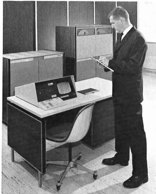
Ampex engineer observing Videofile System as applied to storing, retrieving and displaying scientific data.
